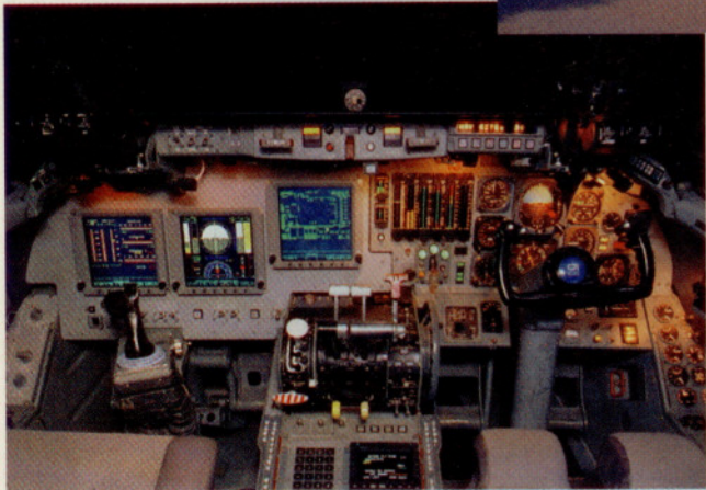
Each Space Shuttle pilot trains in a Gulfstream II Shuttle Training Aircraft (STA) (right). The G-II cockpit, with the left seat set up as it would be in the shuttle. (below).
