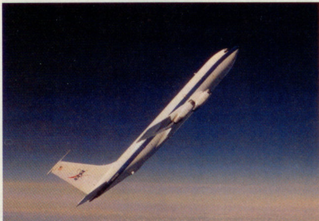
The zoom climb of 350 knots at a 45-degree nose-high angle earned NASA's KC-135A its nickname, the "Vomit Comet."
