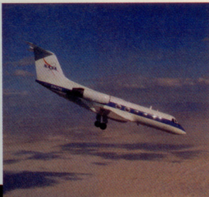
Each Space Shuttle pilot trains in a Gulfstream II Shuttle Training Aircraft (STA) (right). The G-II cockpit, with the left seat set up as it would be in the shuttle. (below).
